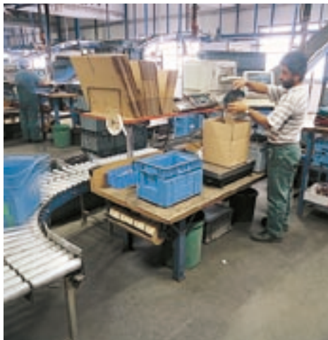
METTLER TOLEDO parts counting systems monitor Production and record the results on a printer or the computer system.
