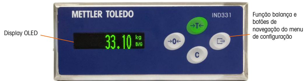
Figura 1-9: Layout de painel frontal IND331
