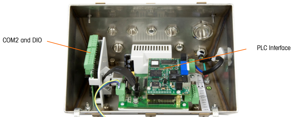
Figure 2-43: Option Locations in the Harsh Enclosure
