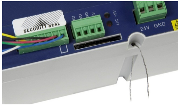
Figure 2-82: DIN and Panel-Mount Sealing – Wire and Paper Seals
