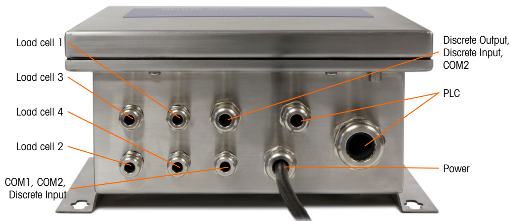
Figure 2-26: J-Box Enclosure Gland Assignments, Original Version
