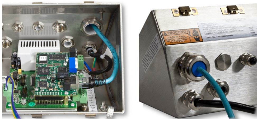
Figure 2-66: Ethernet Cable Routing – harsh Enclosure
