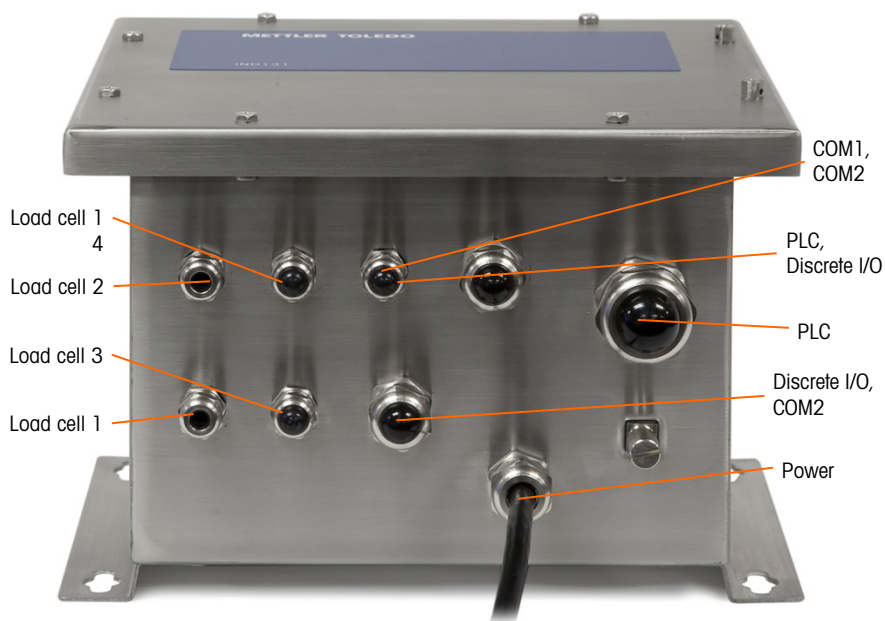
Figure 2-27: J-Box Enclosure Gland Assignments, Updated Version
