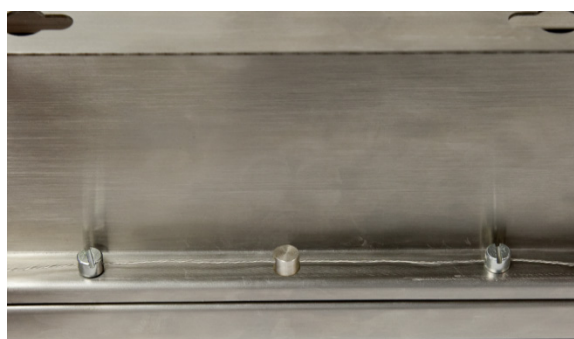
Figure 2-84 : Apposition des sceaux version Junction Box (originale) – Goujon et vis de scellage
