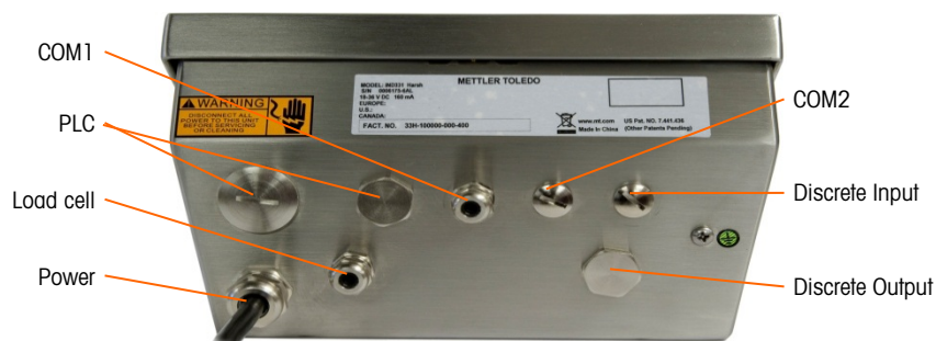
Figure 2-25: Harsh Enclosure Gland Assignments
