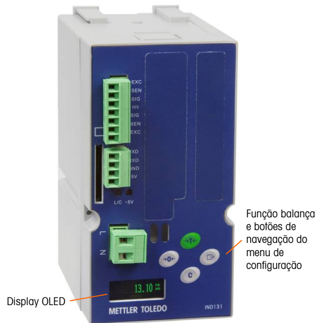
Figura 1-8: Layout de painel frontal IND131
