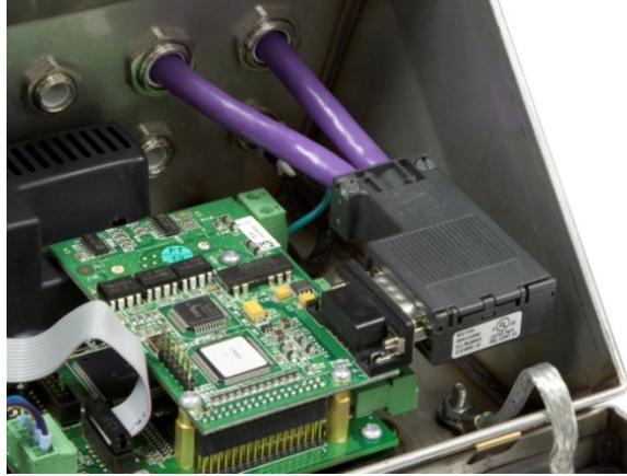
Figure 2-69: Harsh Enclosure PROFIBUS Cable Routing
