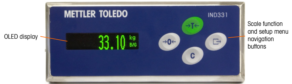
Figure 1-9: IND331 Front Panel Layout
